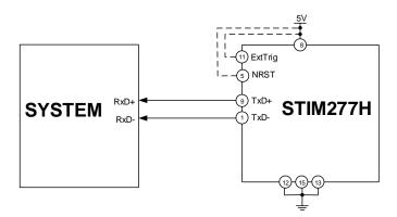
Figure 7-1: Transmit-Only Electrical Connection Diagram
