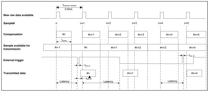
Figure 7-3: Timing of external trigger
