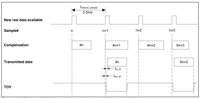
Figure 7-4: Timing of TOV (example: sample rate = 1000samples/s)
