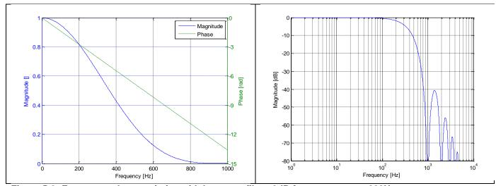
Figure 5-9: Frequency characteristics with low-pass filter -3dB frequency set to 262Hz
