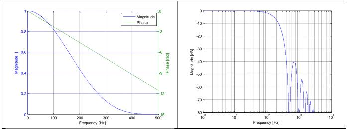
Figure 5-8: Frequency characteristics with low-pass filter -3dB frequency set to 131Hz
