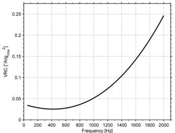
Figure 5-1: Nominal VRC at 20g rms for gyros (ref. section 6.2 for sensitive directions to acceleration-forces)
