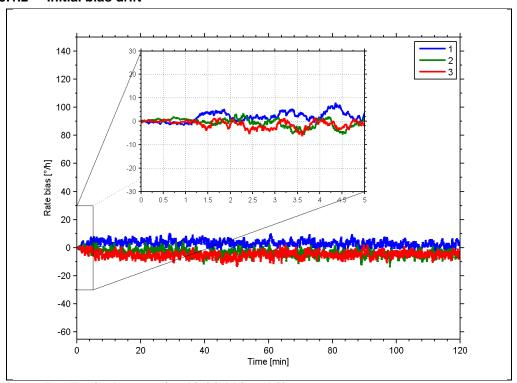
Figure 5-3: Typical normalized initial bias drift
