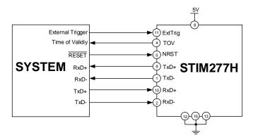
Figure 7-2: Full Function Electrical Connection Diagram
