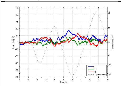
Figure 5-4: Typical Bias drift over temperature
