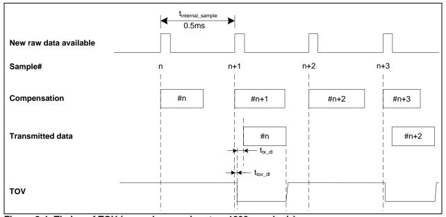
Figure 8-4: Timing of TOV (example: sample rate = 1000samples/s)
