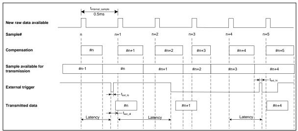
Figure 8-3: Timing of external trigger
