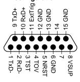
Figure 7-3: Pin configuration as seen from front of STIM318
