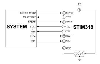
Figure 8-2: Full Function Electrical Connection Diagram
