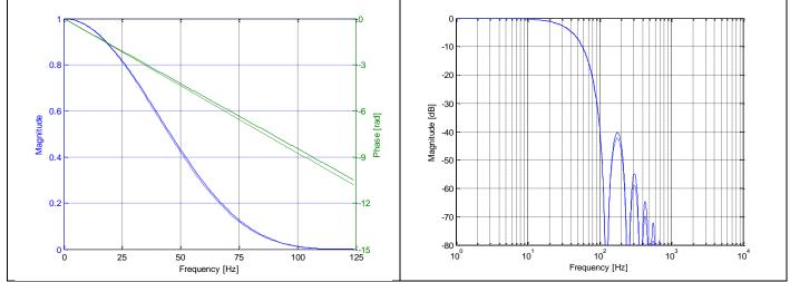
Figure 6-14: Frequency characteristics of accelerometers with low-pass filter -3dB frequency set to 33Hz (solid line: nominal, dashed line: minimum bandwidth, limited by accelerometer)
