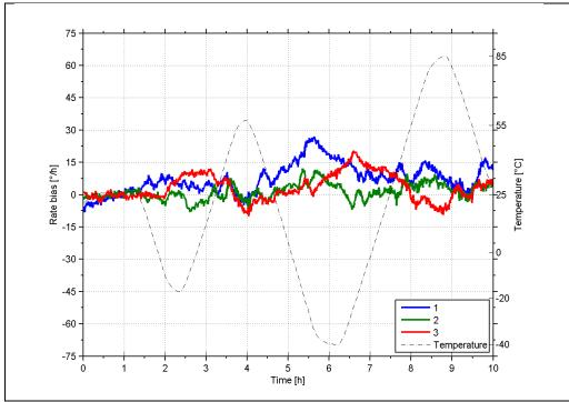
Figure 6-5: Typical Bias drift over temperature (400°/s gyro)
