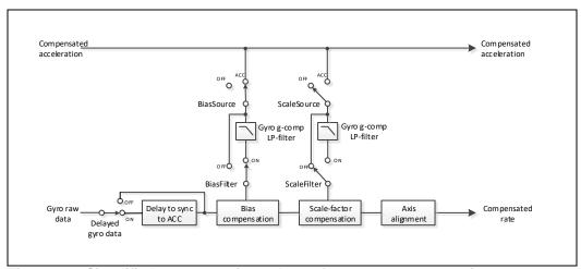
Figure 8-9: Simplified compensation-scheme for gyro g-compensation
