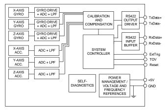
Figure 2-1: STIM318 FUNCTION BLOCK DIAGRAM
