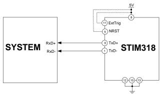
Figure 8-1: Transmit-Only Electrical Connection Diagram
