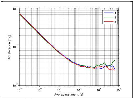
Figure 6-11: Typical Allan-Variance of accelerometer (10g accelerometer)
