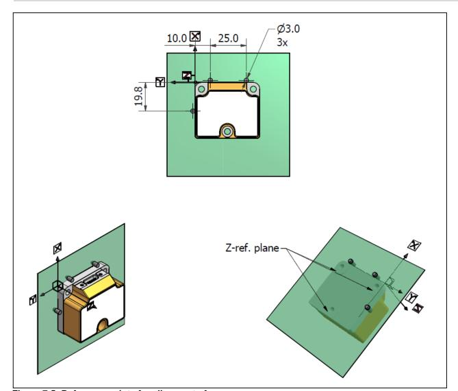
Figure 7-5: Reference points for alignment of axes
