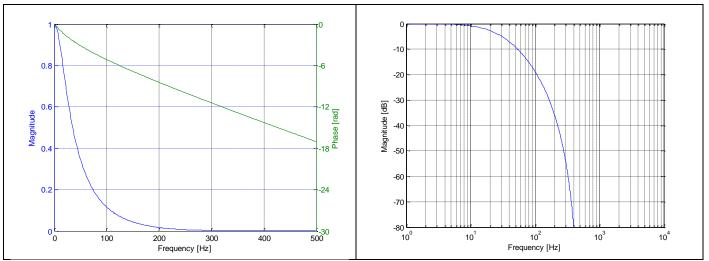
Figure 5-23: Frequency characteristics of inclinometers with low-pass filter -3dB frequency set to 131Hz
