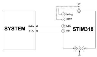
Figure 7-1: Transmit-Only Electrical Connection Diagram
