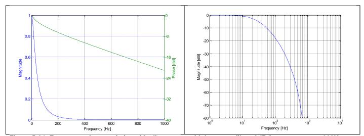
Figure 5-24: Frequency characteristics of inclinometers with low-pass filter -3dB frequency set to 262Hz
