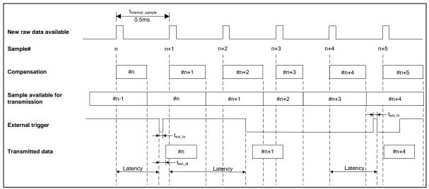
Figure 7-3: Timing of external trigger
