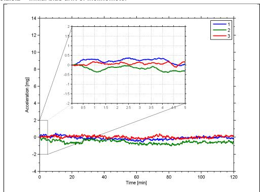
Figure 5-19: Typical normalized initial bias drift of inclinometer
