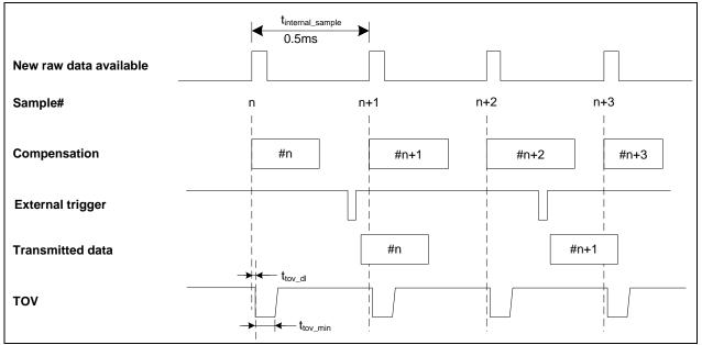
Figure 7-5: Timing of TOV with external trigger
