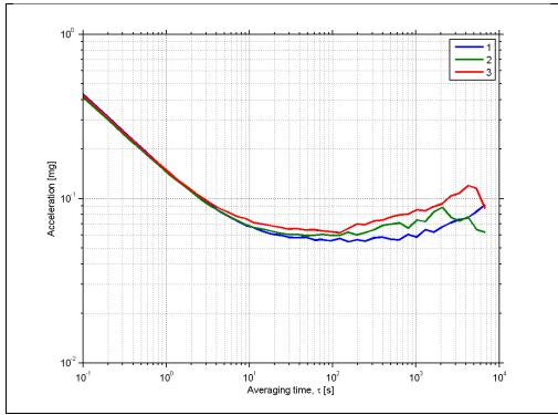
Figure 5-18: Typical Allan-Variance of inclinometer
