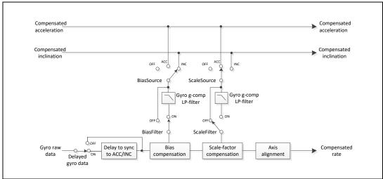
Figure 7-9: Simplified compensation-scheme for gyro g-compensation
