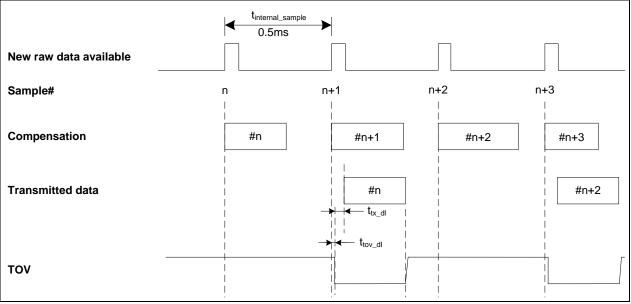
Figure 7-4: Timing of TOV (example: sample rate = 1000samples/s)
