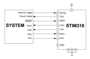
Figure 7-2: Full Function Electrical Connection Diagram
