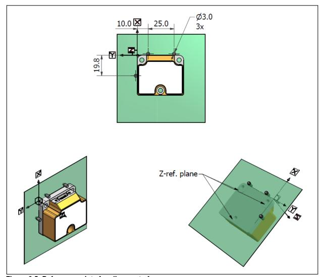
Figure 6-5: Reference points for alignment of axes
