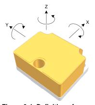
Figure 6-4: Definition of axes
