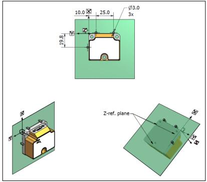
Figure 6-1: Reference points for alignment of axes
