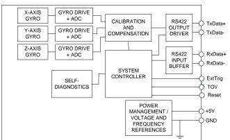
Figure 2-1: STIM210 FUNCTION BLOCK DIAGRAM
