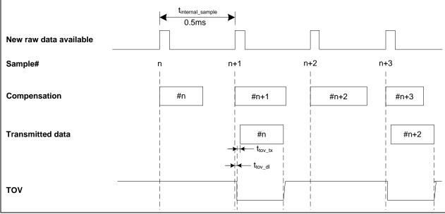
Figure 8-4: Timing of TOV (example: sampling rate = 1000samples/s)
