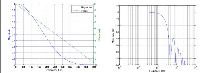
Figure 6-9: Frequency characteristics with low-pass filter -3dB frequency set to 131Hz
