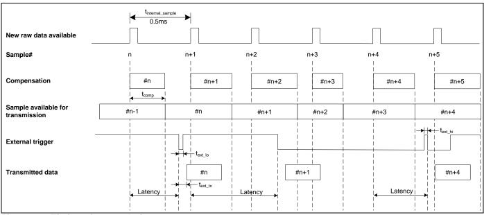
Figure 8-3: Timing of external trigger
