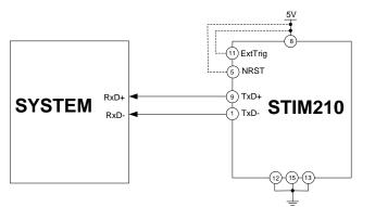
Figure 8-1: Transmit-Only Electrical Connection Diagram
