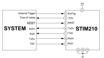
Figure 8-2: Full Function Electrical Connection Diagram
