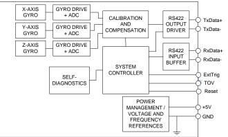
Figure 2-1: STIM210 FUNCTION BLOCK DIAGRAM
