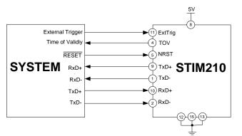
Figure 8-2: Full Function Electrical Connection Diagram
