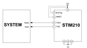
Figure 8-1: Transmit-Only Electrical Connection Diagram
