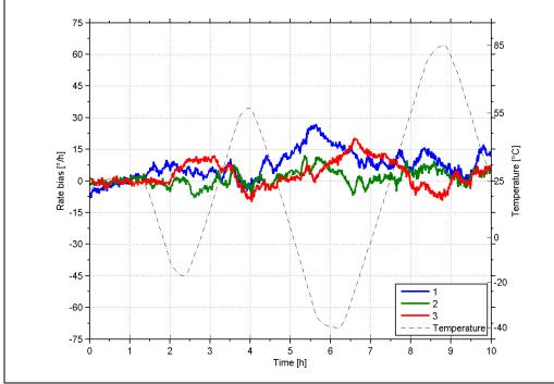
Figure 6-5: Typical Bias drift over temperature
