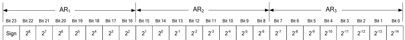
Figure 8-7: Converting output bytes to [°/s]
