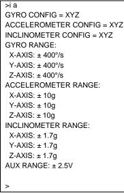
Figure 10-5: Example of response from i a (INFORMATION on AXIS CONFIGURATION) command
