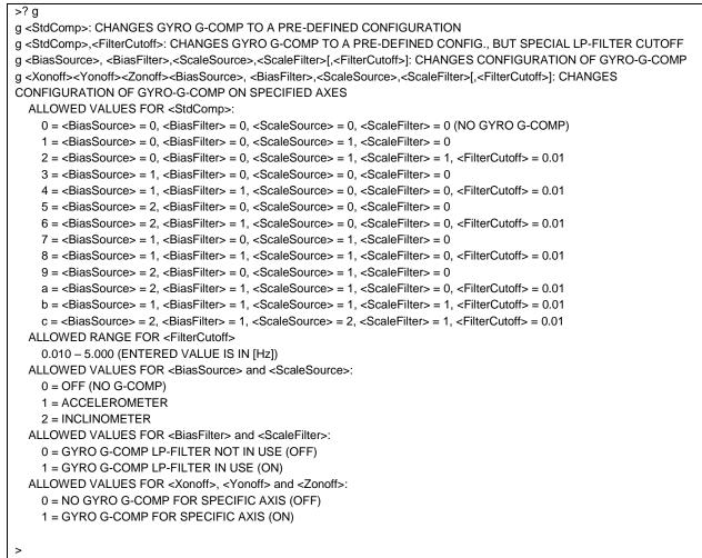
Figure 10-60: Example of response from ? g (HELP on GYRO G-COMP) command
