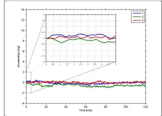
6.1.3.2 Initial bias drift of inclinometer
