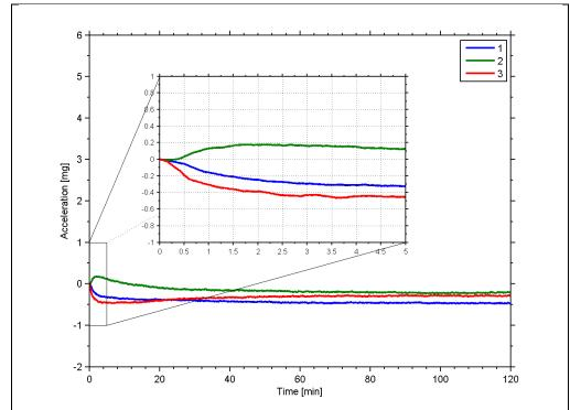
6.1.2.2 Initial bias drift of accelerometer
