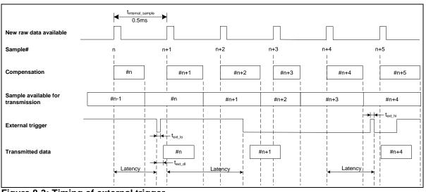
Figure 8-3: Timing of external trigger
