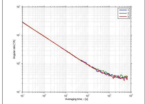
Figure 6-4: Typical Root Allan-Variance of gyro (400°/s gyro)
