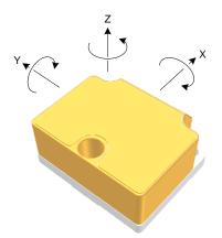
Figure 7-4: Definition of axes
