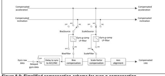
Figure 8-9: Simplified compensation-scheme for gyro g-compensation
