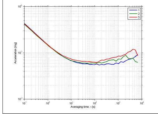
Figure 6-19: Typical Allan-Variance of inclinometer
