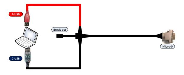
Figure 7: Connecting the EVK to a computer.
