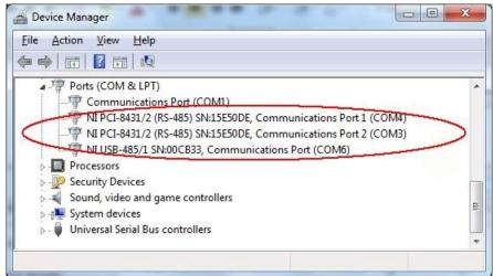
Figure 6: COM port assignments for PCI/PCIe card cable in Windows 7
