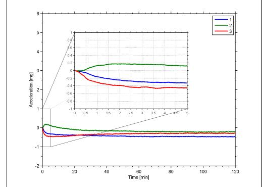
Figure 5-12: Typical normalized initial bias drift of accelerometer (10g accelerometer)
