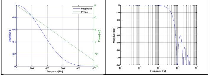
Figure 5-10: Frequency characteristics of gyros with low-pass filter -3dB frequency set to 262Hz
