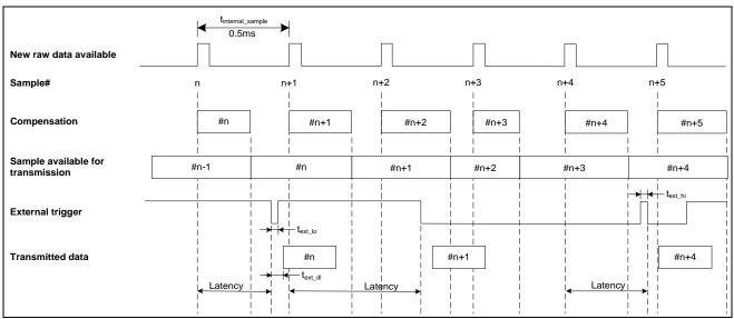
Figure 7-3: Timing of external trigger
