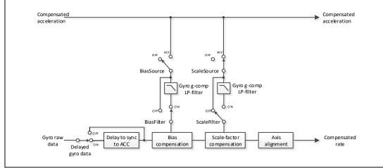
Figure 7-12: Simplified compensation-scheme for gyro g-compensation
