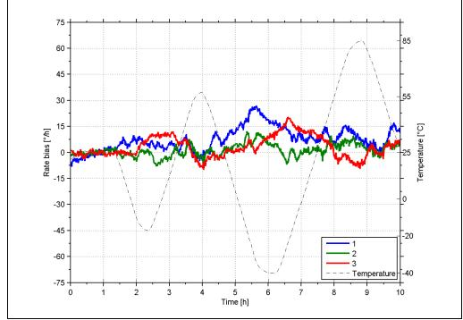
Figure 5-5: Typical Bias drift over temperature (400°/s gyro)
