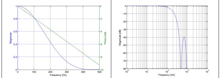
Figure 5-21: Frequency characteristics of PPS filtered with low-pass filter -3dB frequency set to 131Hz
