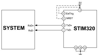
Figure 7-1: Transmit-Only Electrical Connection Diagram
