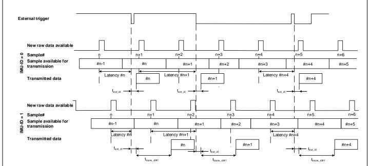
Figure 7-4: Timing of external trigger and multi-module transmission
