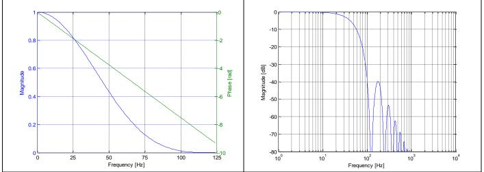
Figure 5-19: Frequency characteristics of PPS filtered with low-pass filter -3dB frequency set to 33Hz
