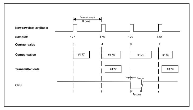
Figure 7-8: Timing of CRS (example: sample rate = 1000 samples/s, counter interval = 5)
