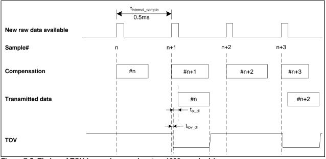
Figure 7-5: Timing of TOV (example: sample rate = 1000samples/s)
