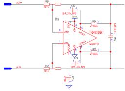
Figure 5-3: AUX input circuitry
