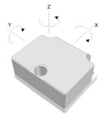
Figure 6-4: Definition of axes
