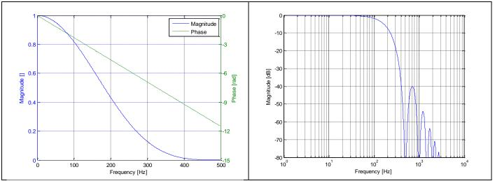
Figure 5-10: Frequency characteristics of gyros with low-pass filter -3dB frequency set to 131Hz
