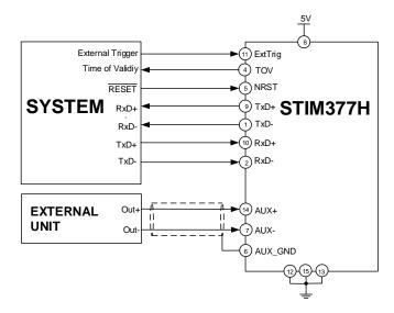
Figure 7-2: Full Function Electrical Connection Diagram
