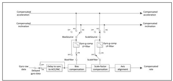
Figure 7-9: Simplified compensation-scheme for gyro g-compensation
