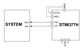
Figure 7-1: Transmit-Only Electrical Connection Diagram
