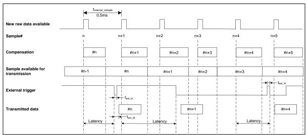
Figure 7-3: Timing of external trigger
