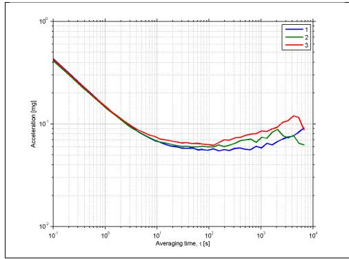
Figure 5-19: Typical Allan-Variance of inclinometer
