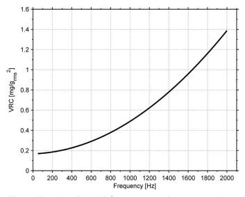
Figure 5-2: Nominal VRC at 10g rms for 10g accelerometers
