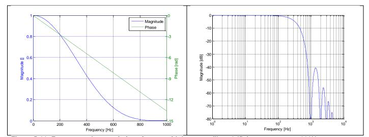
Figure 5-11: Frequency characteristics of gyros with low-pass filter -3dB frequency set to 262Hz
